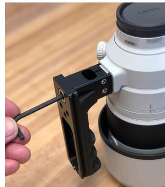
**3.** Insert the long bolt into the bottom of the Big Grip and use the Allen key provided to turn and engage the threaded hole in the lens collar. You may need to slide the Big Grip on the dove tail a small amount back and forth for the bolt to find the hole. It should screw in easily. If any binding is felt STOP and restart the process.
