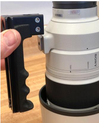
**2.** Do a trial fit of the Big Grip on the male dovetail of the lens collar. It should slide on easily or with a very modest push. The 1/4-20 threaded hole in the lens collar needs to line up with the screw hole in the Big Grip pedestal.
