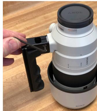
**4.** Using the mid size Allen key, snug up the two side clamp screws until any perceived looseness of the Big Grip on the lens collar goes away. Lightly tighten one, then the other. Do a final tighten on the first then the second.
